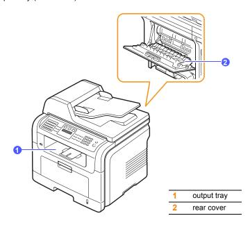
The printer sends output to the output tray by default. To use the output tray, make sure that the rear cover is closed.
